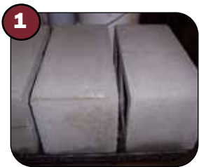
Test samples of silicate left on concrete.
