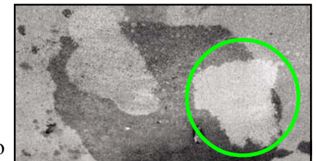
GSR was used on the area inside the circle on this oil stain on a concrete floor.
